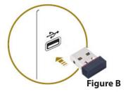
Install the Micro USB receiver (Figure B) into a USB port on the computer or into any of the USB ports on the charging station and wait for the device to Plug and Play. Your Seal Shield™ mouse is designed to use the default drivers on your computer, so no additional software is necessary.
